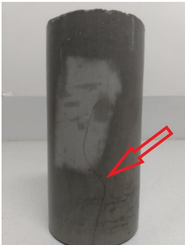
**Figura 35: Rachadura destacada no CP-0F14D.**
